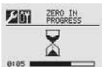
Figure 44. Zero Calibration in Progress
